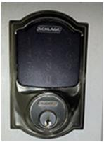
When you push, "Schlage" the keypad will light up in blue. After you push Schlage and then your 4 numbers you will see a green check mark at the lower left side of the keypad. When the motor sound stops, turn the handle and open the door.
